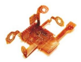
Flex circuits make electronic interconnection both simpler and more reliable. They translate the advantation of manufactures single-layer circuits, double-layer circuits, multilayer circuits, rigid-flex and Flex-Coi Flex circuits can be shaped to fit where no other design can. They are a hybrid of ordinary printed circuits.
